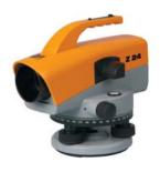
As a rule of thumb, the magnification should be the target distance in metres. Levels with a 24x magnification are ideal for applications on the construction site. Levels with a 28x or 32x magnification are used mainly for engineering and surveying purposes.
